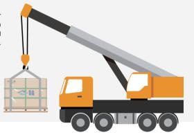
When the crane is used to unload, please use special tooling. Before lifting, please choose a lifting tool with sufficient tension according to the weight and size of the module, and adjust the position of the sling to keep the center of gravity of the module smooth. Please operate the spreader at an even speed, and hold the carton gently on a relatively flat position when the lifting is close to the ground.
