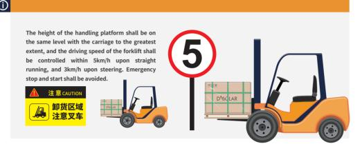
If the packing case shields the view of the forklift driver, the driver is advised to reversely run the forklift during the handling process, and a specialized person shall be assigned to monitor and provide guidance, so as to prevent collision with any persons or articles and avoid injury accidents or damage of the Module due to drop of the packing case. After transporting the packing case the installation site, please place it on the level and hardened ground.
